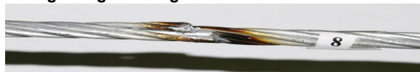
After the lightning discharge and after the vibration tests
