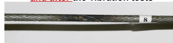
After the lightning discharge and after the vibration tests
